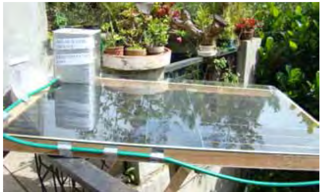
Solar water heat giving 64° Celsius, one of PP Helmut's inventions.
